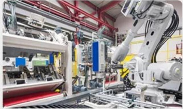
Robot spray mould release agent and
