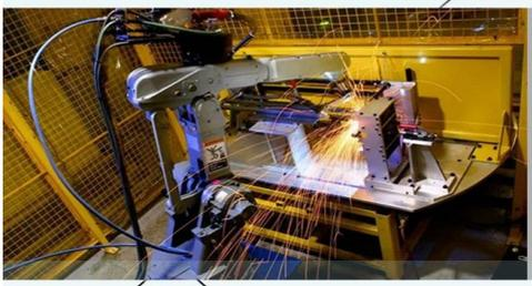
Since 2016, Finehope has continued to purchase welding robots and automatic fixture turntables for welding metal parts. The independent processing of accessories saves the waiting time and procurement cost of outsourcing processing.
