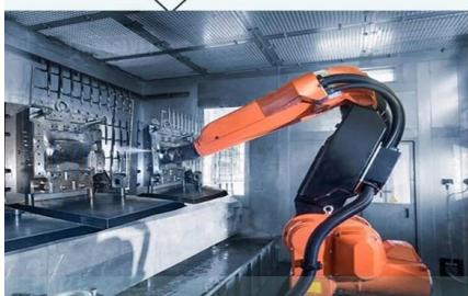
Since 2019, Finehope has purchased robots for spraying water-based release agents to improve the working environment, improve spraying quality and material utilization, and reduce labor costs.
