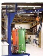
• PU Foaming Equipment (PU发泡器) 发泡设备
